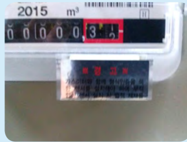
2. Where to insert reed switch.
